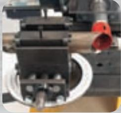
Quick-adjust mitering device
