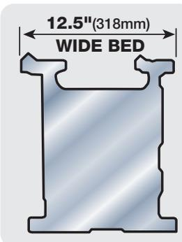
Extra heavy-duty 12.5" (318mm) wide bed gives our machines the capability of withstanding heavy use and excellent durability with minimum maintenance over many years.
