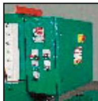
Standard features for the LM1010 control box include: selection for continuous or single cutting stroke, and jog button with reverse switch. A "GO TO" back gauge control pad with stroke counter allows quick, accurate back gauge positioning up to 30 inches.
