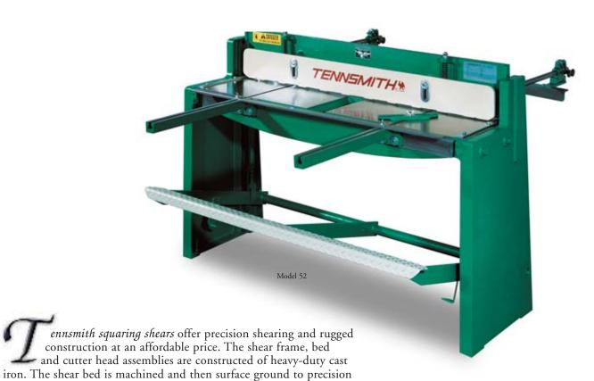
These shears feature triaction, ground-alloy tool steel blades. Both the upper and lower blades have a 2° edge relief and the lower blade has an additional 1° face relief for maximum material penetration with minimum effort. Triaction blades help prevent material movement while shearing, prolonging blade life.
