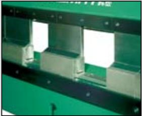
TENNSMITH's new EBT Series is a versatile machine that allows for the removal and repositioning of both the upper and lower segments for forming complex parts. In
