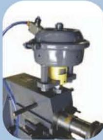
2. Air Over Oil Hydraulic Cylinder - Incremental control with two position foot switch.
