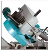
The CT 350 Series Machines are high speed circular saws for aluminum extrusions and other non-ferrous materials. These machines feature swiveling capability for mitering and swiveling/tilting capability for compound mitering.
