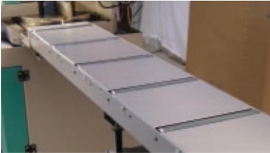
Custom worktable/conveyor w/micro-adjustable legs, mounted to machine.
