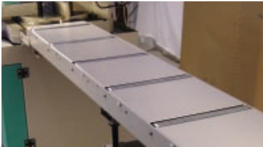
Custom worktable/conveyor w/micro-adjustable legs, mounted to machine.
