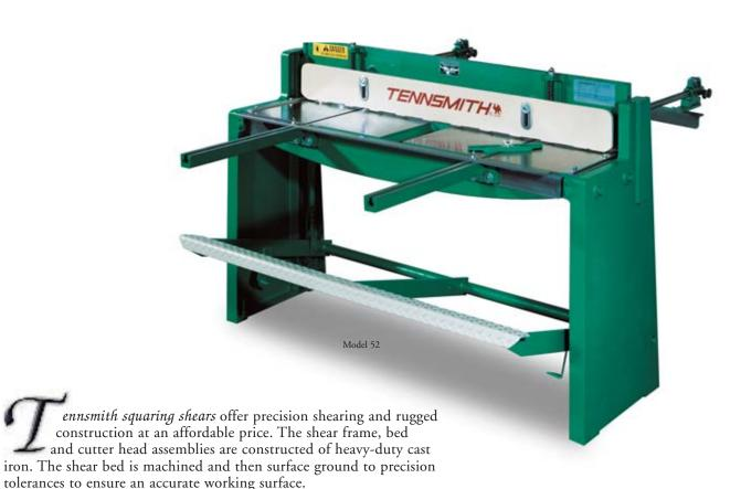
These shears feature triaction, ground-alloy tool steel blades. Both the upper and lower blades have a 2° edge relief and the lower blade has an additional 1° face relief for maximum material penetration with minimum effort. Triaction blades help prevent material movement while shearing, prolonging blade life.
