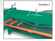
Unlike competitive front return systems, with the LM Series Performance Package F, you can cut materials longer than the standard back gauge length by deactivating the sheet support.
