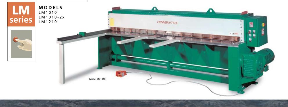
TENNSMITH's LM1010 is equipped with a standard "GO TO" 30-inch back gauge system. The ballscrew-driven back gauge provides quick, accurate cuts. The LM1010 is powered by a 12-1/2-hp gear motor attached to a mechanical linkage which provides smooth, quiet operation.
