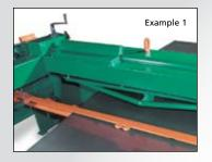
The optional sheet support system is recommended for gauging of thin material. With this air-powered support mechanism, one operator can effectively shear cumbersome, light-gauge stock. The sheet support system is available in two styles: **System F**, available on models LM1014 and LM1214, is a front return support which drops sheared parts to a front chute for easy retrieval; and support **System R** which drops sheared material to the rear of the machine.
