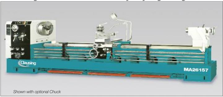
The Clausing MA series large swing geared head engine lathes are engineered to allow the accurate and efficient machining of large components. A wide range of optional accessories make these machines suitable for most industrial applications, including job shops, oil field, power utilities and ship building.
