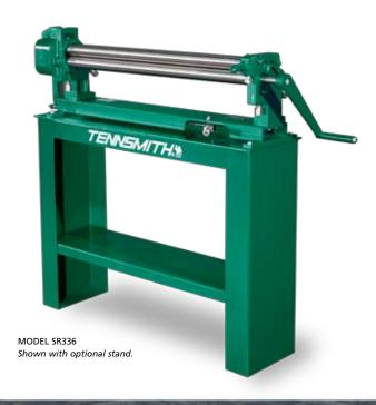
TENNSMITH's slip rolls combine precision-turned, ground and polished high carbon steel rolls with heavy-duty, cast iron end frames and a welded steel base to make an accurate and durable forming tool. Convenient operating features include large roll adjusting screws, scales for speeding repeat set-up, and a front-mounted handle to lift the upper roll for material removal. Wire grooves are standard.
