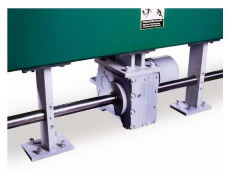
For maximum hemming capacity, another strong feature of the Tennsmith SBS Series is the center drive of the clamping system. The placement of the motor in the center of the machine maximizes power while reducing torque loss through the drive shaft. The benefit is a hemming capacity of 20 gauge for the SBS12614 and 22 gauge for the SBS15016.
