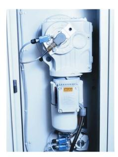
The SBS incorporates a twin motor drive system for the folding beam. This allows the system to be fast and extremely accurate. Bending speeds up to 90 degrees per second can be easily achieved. Another advantage to this system is maintenance. Unlike with chain drive designs, there are no adjustments needed to this direct drive system.
