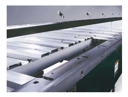
The support panels can be move back to allow gauging of parts with a down flange inside the machine (Z Bar etc.)
