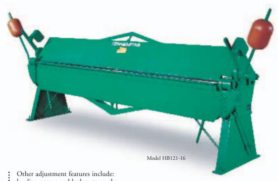
Other adjustment features include: leveling screws and lock nuts on the pedestals; jack screws and tensioner bolts on the apron; truss rods on the apron, base, and upper leaf; and fully adjustable counter balances to facilitate the bending process. Removable apron angle and insert permit 1/4-inch reverse bends in lighter material.
