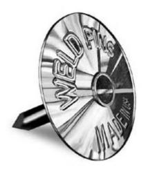
PowerPoint weld pins are used to fasten insulation to the inside of sheet metal air ducts. These fasteners are usually applied when the ductwork is being fabricated. The fasteners have been specifically designed to work with all currently available duct liners and standard resistance welding type application equipment.
