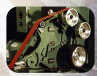
Part No. 1277 2" Fork Arm 2" wide yoke attachment. 2" x 72" belt, Wheel dia. 9/16", 3/4", 1", 1-1/2"
