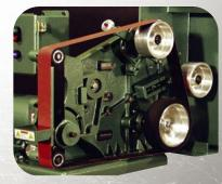
Part No. 1274 Yoke attachment with standard 2" x 2" contact wheels. Backup platen is removable for contour and loose belt grinding.
