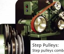
Step pulleys combined with optional size drive wheels allows 16 different speeds ranging from 677 S.F.P.M. to 6320 S.F.P.M.
