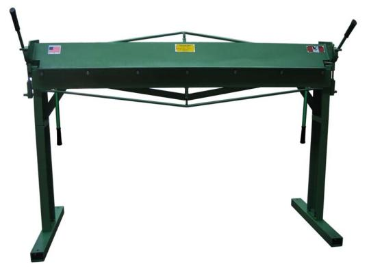
The TK 622 Straight Brake, 6' x 22 Ga. GREAT FOR CROSS BRAKING 4' DUCT!
