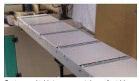
Custom worktable/conveyor w/micro-adjustable legs, mounted to machine.
