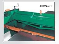
The optional sheet support system is recommended for gauging of thin material. With this air-powered support mechanism, one operator can effectively shear cumbersome, light-gauge stock. The sheet support system is available in two styles: **System F**, available on models LM1014 and LM1214, is a front return support which drops sheared parts to a front chute for easy retrieval; and support **System R** which drops sheared material to the rear of the machine.
