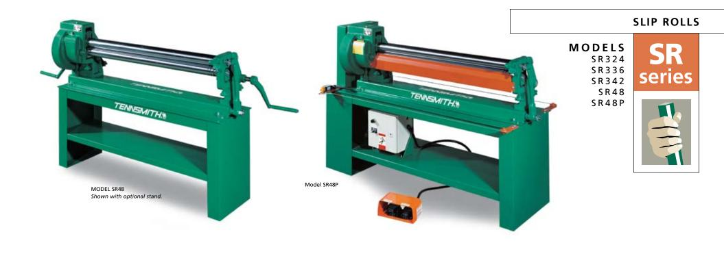
Drive power for the SR48P is supplied by a heavy-duty, industrial quality gear reduction motor and roller chain directly to the gear train. The roll drive is controlled by a toggle action, shrouded foot pedal for instant forward and reverse action. The drive motor is equipped with an electromagnetic brake to prevent roll creep and over-forming.
