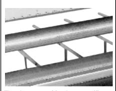
The cleanup position leaves sufficient space between the upper roll and the adhesive roll to allow for easy cleanup without endangering the operator.
