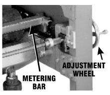
A metering bar accurately controls adhesive application.
