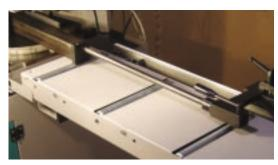
Custom worktable/conveyor with Accu-cut custom length system Stop with scale, micro-adjustable legs 72" and 144" lengths available
