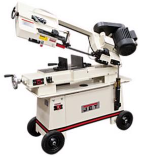
The J-3410 7" x 12" Horizontal Wet Bandsaw is fully equipped with a 3/4HP motor, side and rear blade guides, heavy duty cast iron head and table, and rapid acting vise. The included 3/4" bi-metal blade comes to a stop after each cut with the automatic shutoff.
