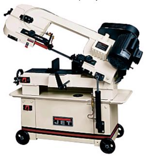
The JET HVBS-7MW Metalworking Bandsaw is UL listed and powered by a 3/4 HP motor. 4 large diameter wheels and built in handle allow easy movement. Each HVBS-7MW comes equipped with a 3/4" carbon steel blade, adjustable material stop and vertical worktable. Worried about safety? Don't – the HVBS-7MW shuts off automatically after each cut.
