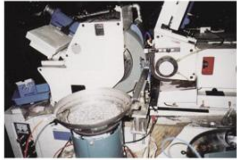
Centerless grinding machine model: JHC-18S with vibratory parts feeder and straight line feeder.
