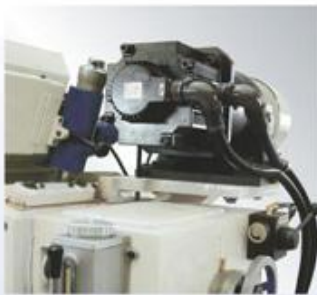
JHC-12S with servo motor for regulating wheel, variable speed.
