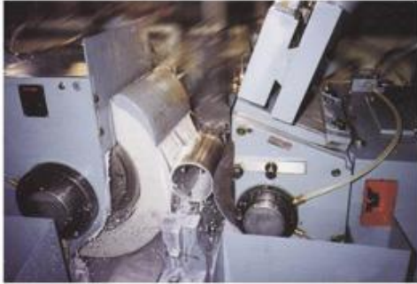
Centerless grinding machine model: JHC-18S with vibratory parts feeder and straight line feeder.
