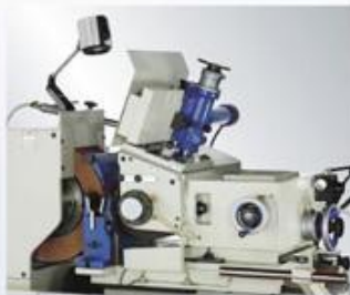
JHC-18 drive with 10 step variable speed
