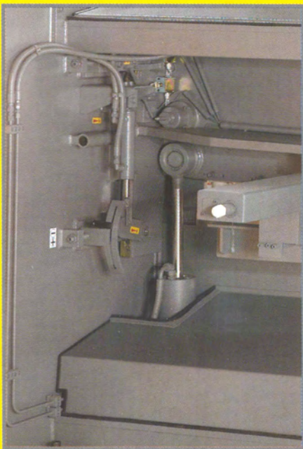
Picture including hydraulic blade gap setting (standard on HDE models with SC70 control unit)
